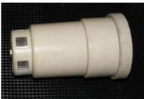
Figure 12. Obsolete smoke detector responsible for elevated gamma-ray dose rate in SW corner of the lecture room..
